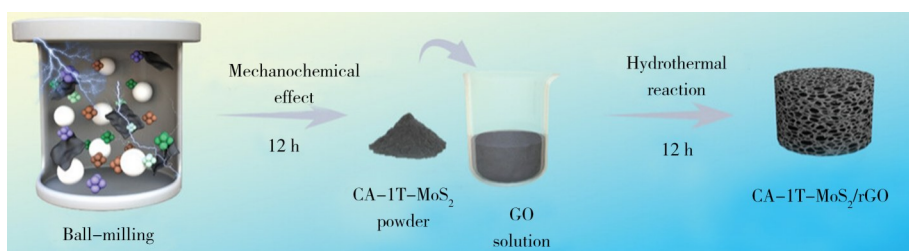
图3 CA-1T-MoS 2 /rGO 的制备示意图 [35] Fig. 3 Scheme of the preparation of CA-1T-MoS 2 /rGO [35]
